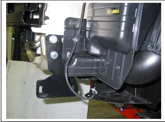
Figure 9 – Passenger side air intake box refitted
