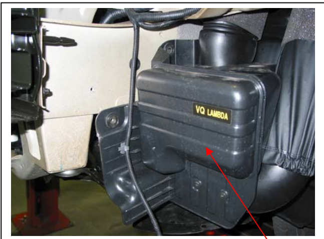
Figure 5 Air box on passenger side moved
