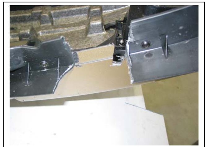
Figure 12 – Driver's side shown with section of lower black trim removed and approximately 40mm into bumper cover for steel mounting plate.
