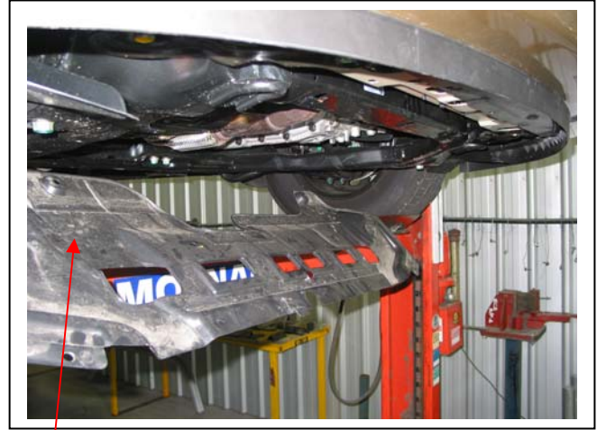
Plastic under guard Figure 4 being removed
