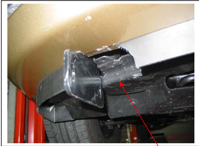
Figure 15 – Driver's side shown Plastic under guard trimmed around steel mounting plate
