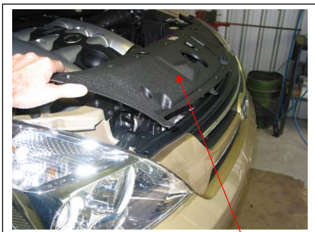
Figure 1 Shown removing plastic cover
